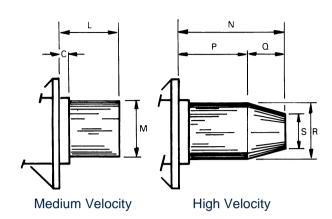
For all MULTIPLEX burners with stainless steel combustion tunnels dimensions given are for standard tunnel length. Tunnels may be extended to suit application requirements. Refractory tunnels can be extended to order.
