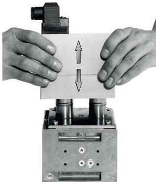
9. Replacing the solenoid Versions with adjusting plate DMV-D 5.../11 or hydraulic brake DMV-DLE 5.../11
