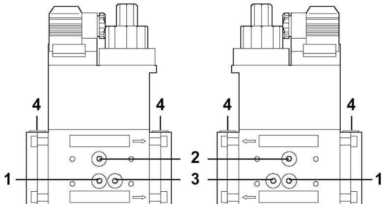
Screw plugs 1,2,3 may also be replaced by a measuring socket G 1/8 DIN ISO 228.
