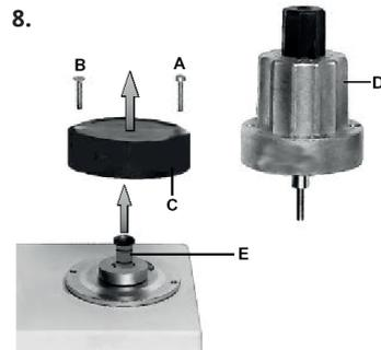
8. Replacing hydraulic brake unit or adjustment plate
