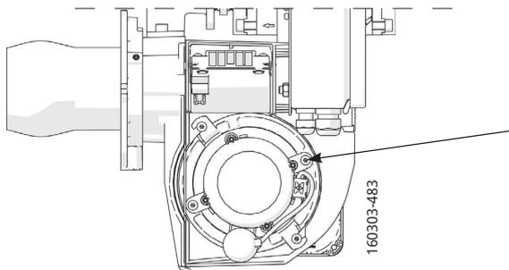
Use screw to attach the vibration sensor.
