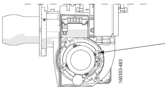
Use screw to attach the vibration sensor.
