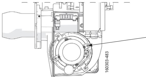
Use screw to attach the vibration sensor.
