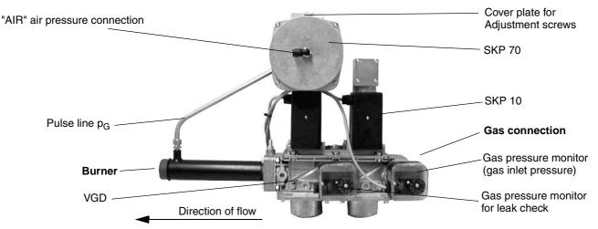
Connect the blue hose to the "AIR" connection on the gas train and the air pressure connection on the gas jacket. The blue hose serves as a control line for the gas train and must be routed in a loose loop without kinking.
