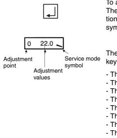
To access the service mode, press the **enter key** for approx. 2 sec. The following now appear on the display: point **P0** and the air flap positioning motor setting value at ignition in angular degrees, plus a wrench symbol denoting the service mode.
