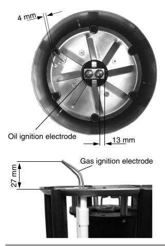
The following clearances between the nozzle and ignition electrode should be observed:
