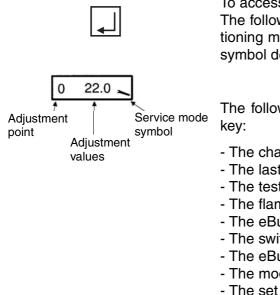
To access the service mode, press the **enter key** for approx. 2 sec. The following now appear on the display: point **P0** and the air flap positioning motor setting value at ignition in angular degrees, plus a wrench symbol denoting the service mode.
