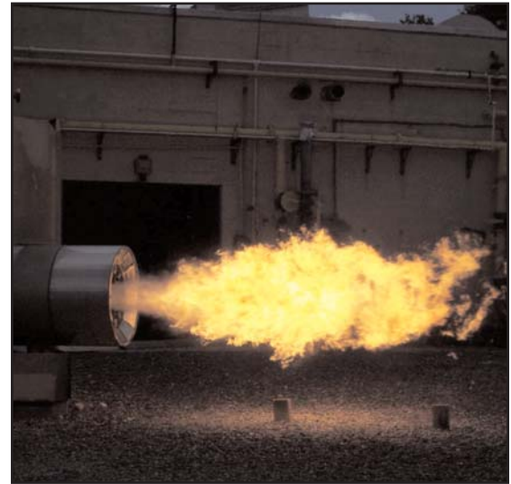
ECO-STAR II 150 High Fire @ 160 MM Btu/hr (42,300 kW) No. 2 Fuel Oil Low Pressure @ Low Spin Setting
